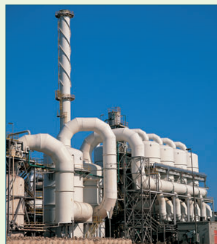
figure ci.5 Heavy insulation prevents the costly loss of heat from a sulfuric acid manufacturing plant.
