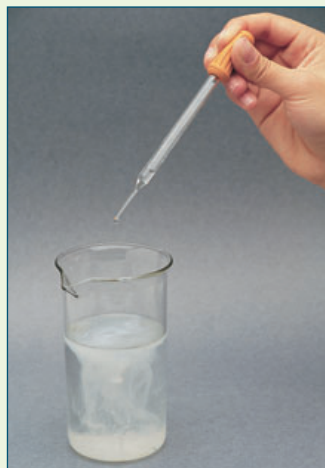
figure fa.3 Precipitation reactions provide simple means for testing for ions, both qualitatively and quantitatively.
