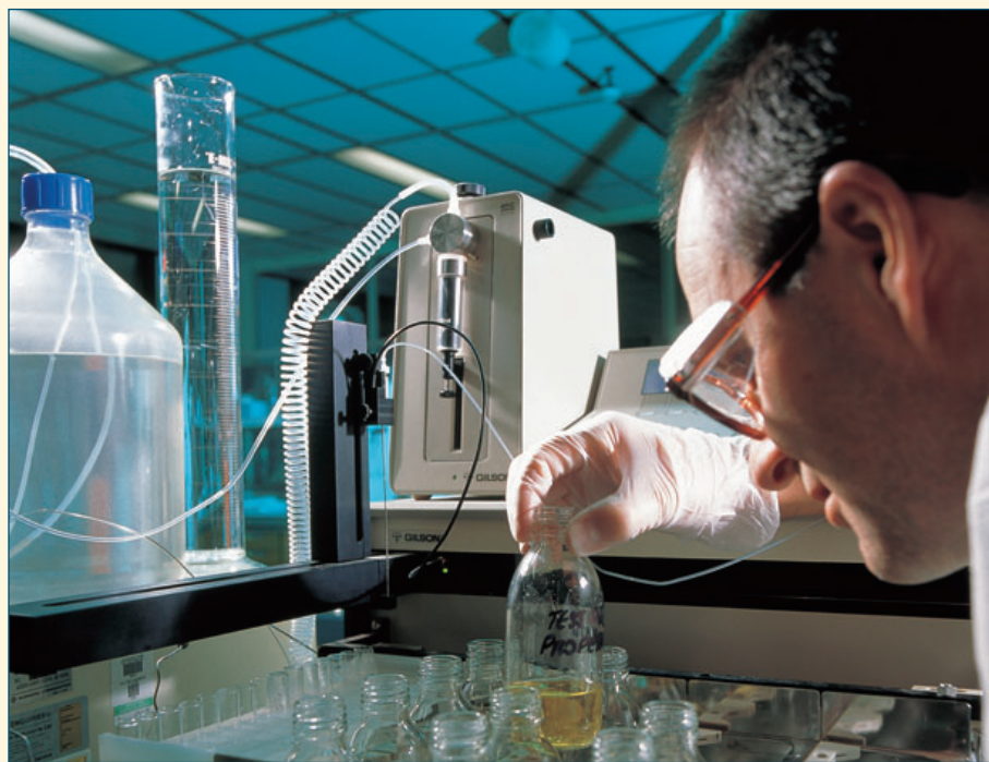
figure qc.3 This scientist is using chromatography to check for pesticides in food.
