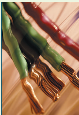
figure ec.3 Copper needs to be very pure to work effectively as an electrical conductor. Copper is refined to approximately 99.98% purity.
