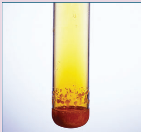
figure cs.10 The liquid bromine produced after leaving the steaming-out tower.
